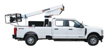
UTLN35A meets and exceeds ANSI A92.2-2015 and OSHA Requirements \*Based on a 35in frame height
